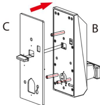
3.2 Insert spindle(H) into the clutch.
