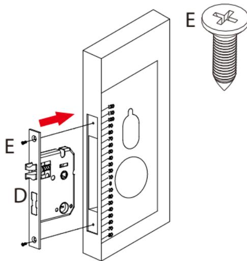
**Note:** Installing the mortise(D) on the door by inserting screws(E).
