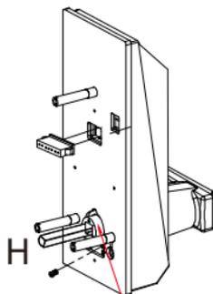
3.3 Attach outdoor unit(B) to door by putting it through door holes.
